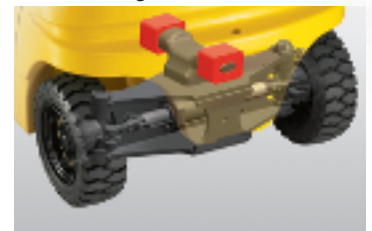
High-mounted Rear Axle
