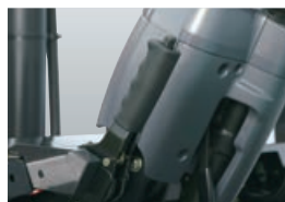
A double acting type brake lever prevents mishandling
